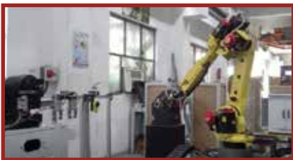
Robot ready to loading/unloading Gear blanks with New gripper set
