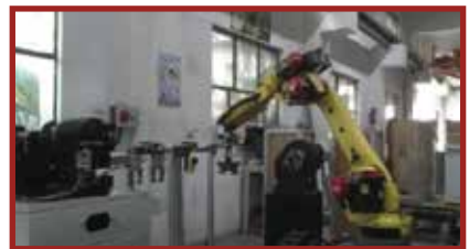
Robot wrist attached to new set of 'Quick change' gripper set for Gear Blank handling.
