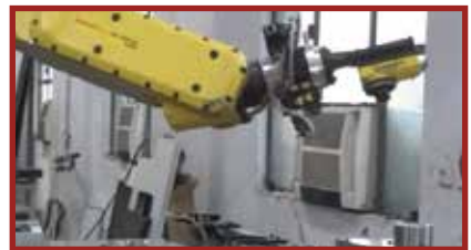
Robot using vision sensor for Inspection.
