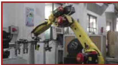
Robot wrist attaching to vision sensor.
